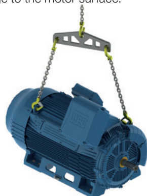
Figure 8 - Lifting with inclined chains.
