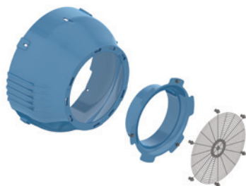
Figure 22 - Mounting system that ensures low noise levels.
